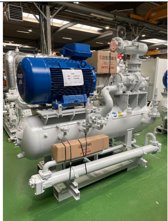
Description: Compressor Skid A (Model No. P160S / Sr. No. 1656466)
