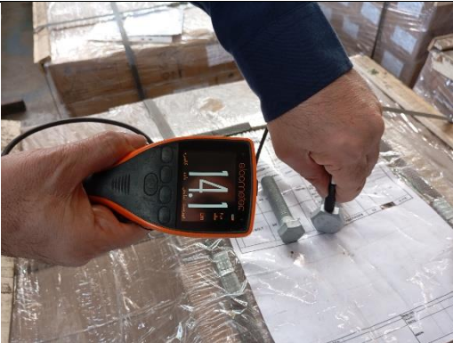
Dacromet coating thickness control
