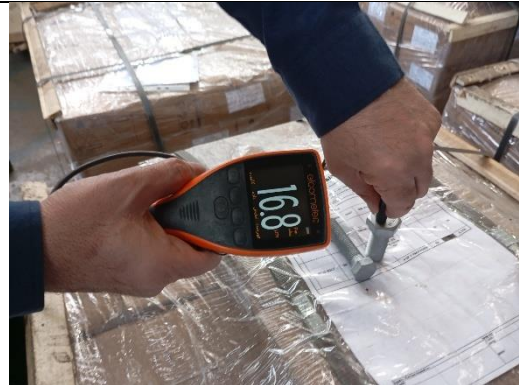
Dacromet coating thickness control
