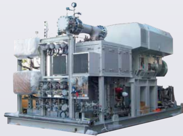
Flare recovery compressor - Saudi Arabia 200M / 700kW
