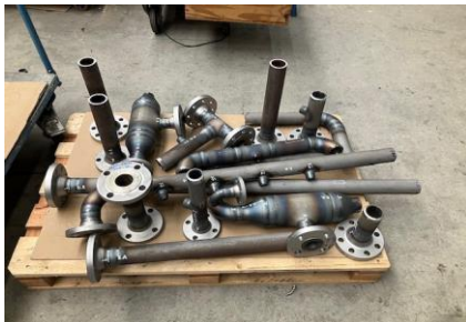
Piping welded ready for inspection
